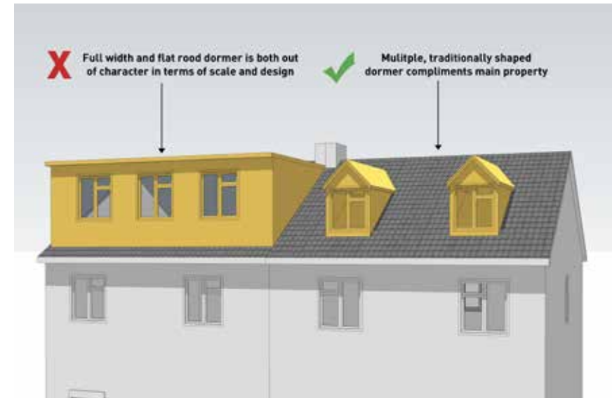
Diagram 9: Large flat roof dormer vs smaller pitched roof dormers
