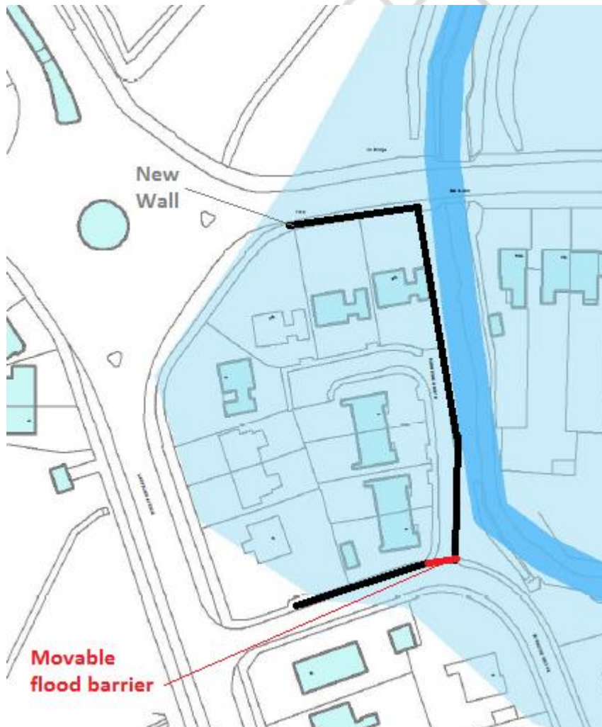
Figure 5: Potential flood solution on Burnside Close
