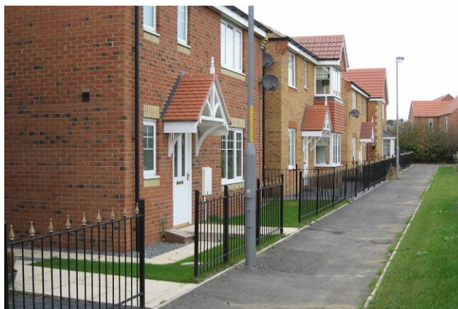
Railings can be used to separate public and private realm and to give privacy to dwellings immediately adjacent to highways.
